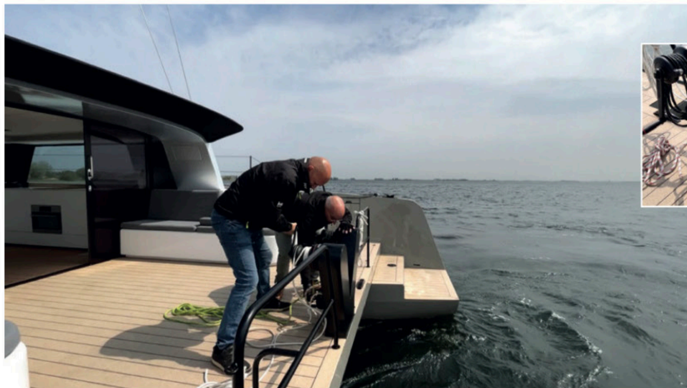
Most of the sail handling maneuvers are carried out on this V-shaped column equipped with two winches.
