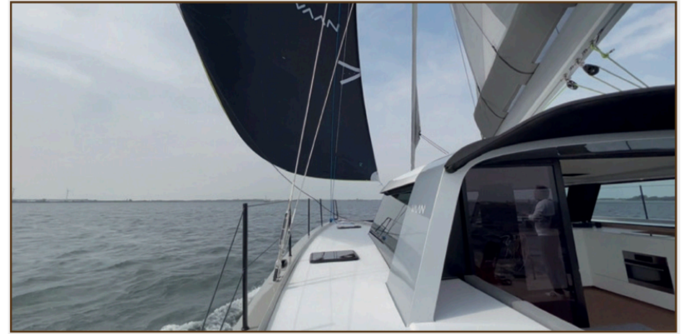
The side-decks are wide and bordered by a decent bulwark, making it safe to move around, though it would be nice to see some handrails added to the coachroof.
