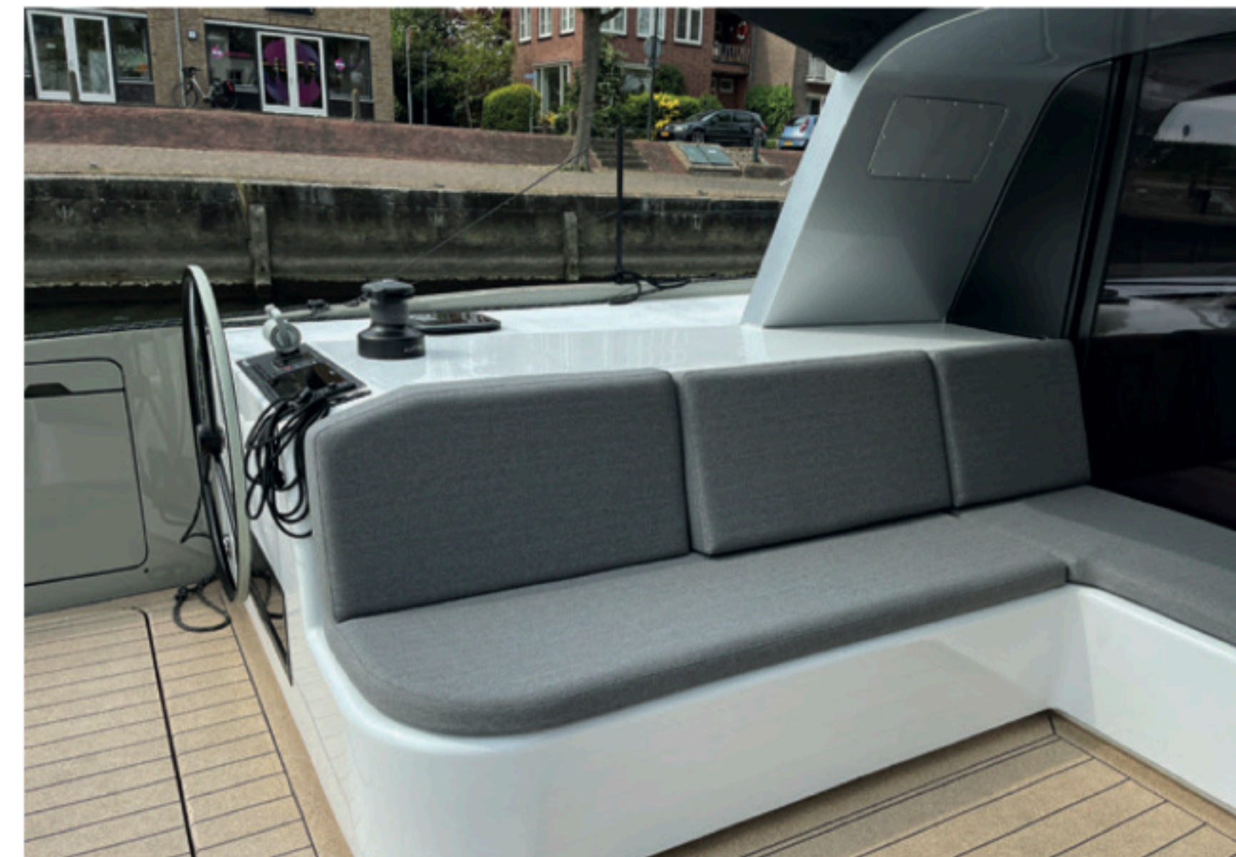
Climbing up on to the side-decks requires using the bench seats as steps (due to the lack of a suitable passageway)... something to be reviewed.
